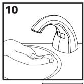
Test the System by passing your hand under the spout of the Dispenser Assembly ①
