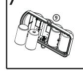
Place four alkaline "D" Cell batteries (not furnished) into the Battery Box (2) cover. The batteries must be positioned according to the diagrams shown on the inside of the cover.
