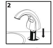
Feed the Data Cable (6) and the shank of the Dispenser Assembly (1) through the hole in the countertop. Point the spout of the Dispenser into the sink bowl and press down firmly on the Dispenser to securely attach it to the countertop.
