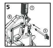
Secure the Motor Assembly/Bottle Support (1) to the Dispenser Assembly (1) shank by pushing the Retaining Clip (5) into place through the vertical slots, until it goes all the way through the Motor Assembly.
