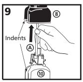
Feed the dispense tube (À) on the Refill Bottle (1) up through the Motor Assembly/Bottle Support (a) and Dispenser Assembly (1), aligning the two indents in the Bottle and the Support. Slide the Bottle upward until it snaps into place.
