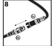
Connect the two halves of the Data Cable (a) and (b) by lining up the white stripes on each half and pushing the cable connectors together until the stripes touch.
