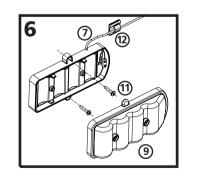
Remove the cover from the Battery Box (1) by loosening the two captive screws on the Battery Box cover. Position the Box on a convenient (vertical or horizontal) surface under the counter top that will allow access for battery changing. Attach the Box to the surface using the two screws (1) and anchors (if attaching to a plaster or masonry surface). Use the Wall Clip (2) to secure the Power Cable (7) to a wall or other under-counter surface if desired.
