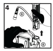
Align the indent inside the top of the Motor Assembly/Bottle Support (18) with the indent on the shank of the Dispenser Assembly (1) and firmly push the Motor Assembly/Bottle Support up, onto the shank.
