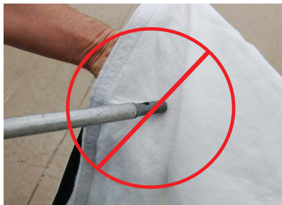
LIGHTLY CLEAN WITH COMPRESSED AIR ONLY, FROM THE OUTSIDE IN. KEEP THE NOZZLE 6-12 INCHES FROM FABRIC
