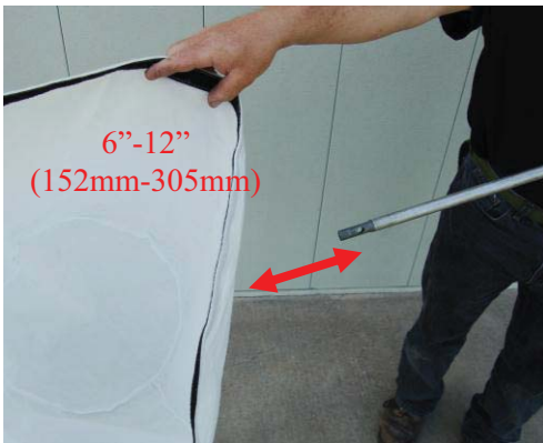
LIGHTLY CLEAN WITH COMPRESSED AIR ONLY, FROM THE OUTSIDE IN. KEEP THE NOZZLE 6-12 INCHES FROM FABRIC
