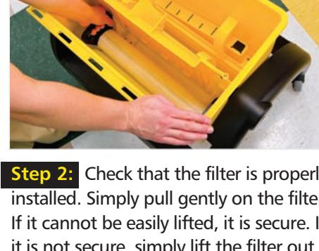
**Step 2:** Check that the filter is properly installed. Simply pull gently on the filter. If it cannot be easily lifted, it is secure. If it is not secure, simply lift the filter out and then reattach by putting the nozzle into the hole and pressing down firmly.
