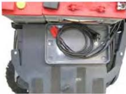
Cable compartment accessible from machine side opening
